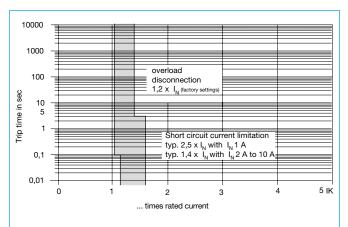
Without the current limitation there would be a much higher overcurrent in the event of an overload or short circuit.
