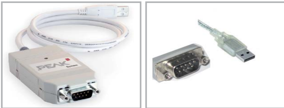
Figure 3: CAN-USB converter cable (example: PEAK)
